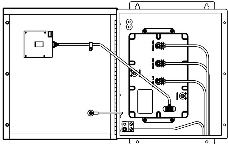
**WIRING DIAGRAM WITH INTEGRAL DISCONNECT**
