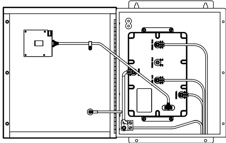
**Figure 3: Three-Phase, 3- or 4-Wire, Grounded Wye Installation**
