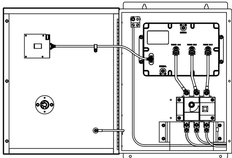
**WIRING DIAGRAM WITH INTEGRAL DISCONNECT**
