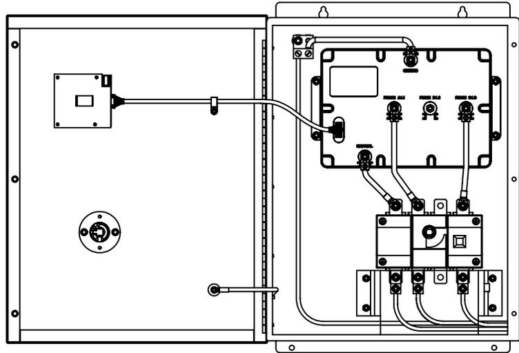
**Figure 9: Three-Phase, 3- or 4-Wire, Grounded Wye Installation with Integral Disconnect**
