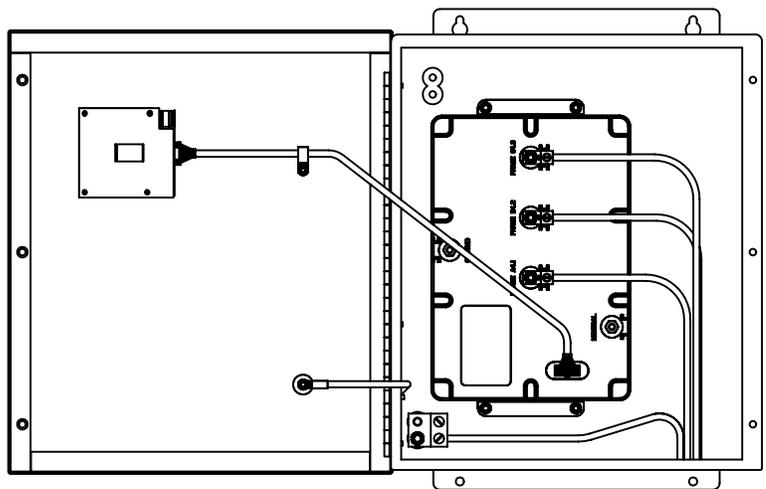
**WIRING DIAGRAM WITHOUT INTEGRAL DISCONNECT**
