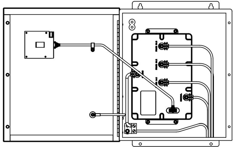
**Figure 5: Three-Phase, 3-Wire, Delta Installation**
